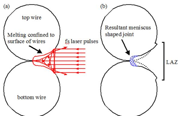
**Figure 6** Proposed mechanism of microweld of the Au crossed wires (a) just before and (b) after fs laser irradiation.
