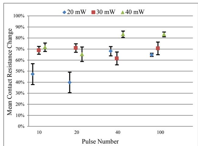
**Figure 5** Average percentage drop in contact resistance of crossed wires as a function of output power with corresponding error bars.
