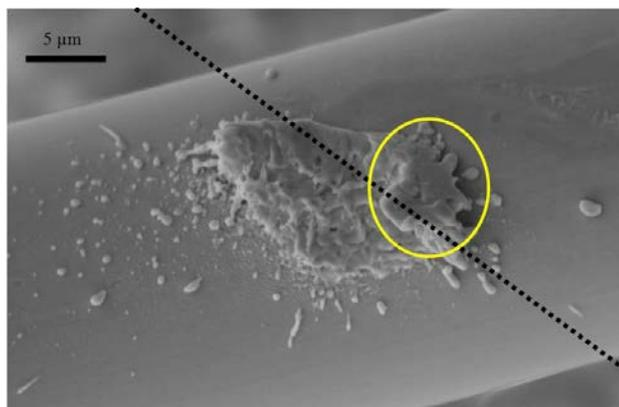
**Figure 7** The LAZ after laser irradiation with  $(P, N) = (30 \text{ mW}, 20 \text{ pulses})$  on the bottom wire. Its length is approximately  $15 \mu\text{m}$ . The proposed meniscus is shown in yellow.
