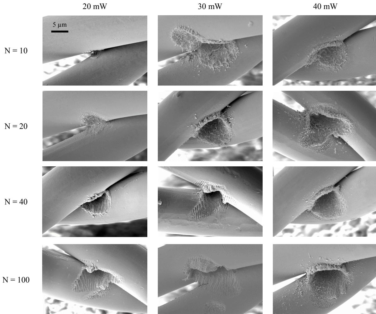
**Figure 4** Weld morphologies as a function of output power and pulse number. Increasing either laser parameter correlate to a greater LAZ between the crossed wires.
