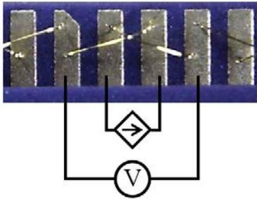
**Figure 2** Schematic diagram of the *in-situ* four-wire contact resistance measurement for one crossed wire sample.
