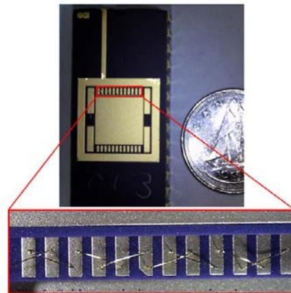
**Figure 1** Gold crossed wires on ceramic substrate. Each substrate houses 8 sets of crossed wires.
