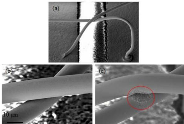
**Figure 3** (a) Overview of a crossed wires sample and close-up of contact point (b) before and (c) after fs laser irradiation. The laser affected zone is outlined in red.
