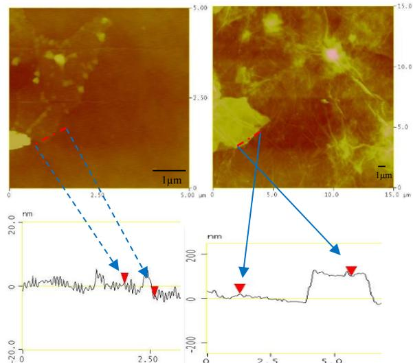
Figure 3: AFM images of diluted rGO solution (left) and as-exposed rGO solution (right). The exposure time, wavelength and laser energy density were 3 hr, 800 nm and  $4.45 \times 10^5 \text{ W/cm}^2$ .
