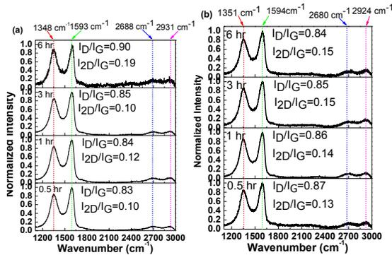
Figure 2: Recorded Raman spectrum of a) as-exposed solutions and b) diluted solutions.
