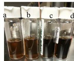
Figure 1: graphene oxide solution after exposed by ultrafast laser ( $\lambda=800$ nm and energy density of  $4.45 \times 10^5$  mJ/cm<sup>2</sup>) for a) 0.5hr, b) 1hr, c) 3hrs and d) 6hrs.
